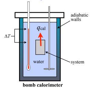
Bomb calorimetry is conducted under constant volume (isochoric) conditions. This is shown explicitly by writing  $q_v$  for the heat term. The subscript "v" means conducted at constant volume. Because the volume is held constant and  $\Delta V$  is forced to be zero, no expansion
